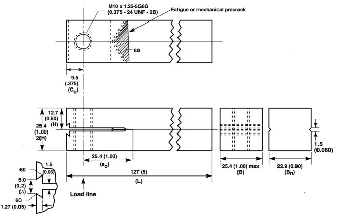
Note 1—All dimensions in mm (in.). Top and front views are shown for smooth specimen only; side view is shown for both smooth and side grooved configuration.
